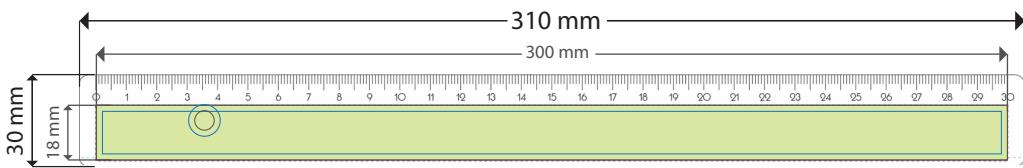
○ Ø 5 mm – POS Mitte 40 mm v. linker Kante, 15 mm v. unterer Kante
